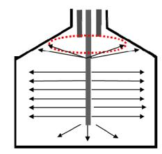
A place where an electrode has high density and has the bestsensiti vity (largeinflue nce of adhesion)
