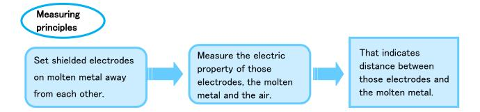
Mystar series does not require an electronic circuit on its electrode head and can be installed in a place away within 300 m. This enables a measurement without influence of a cable's capacitance.
